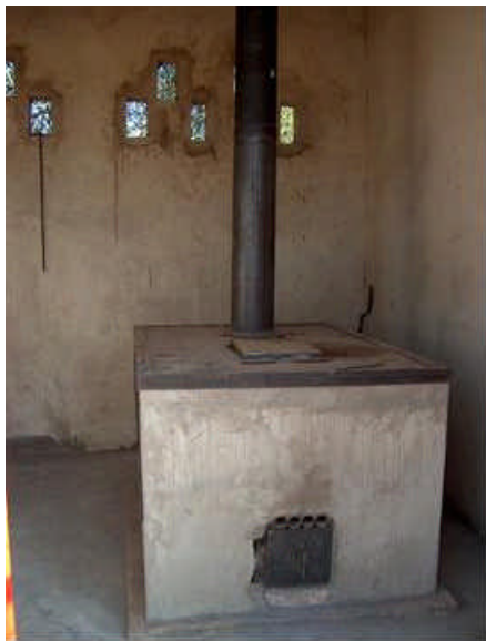
Picture 9: Low cost medical waste incinerator.
