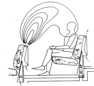
Figure 4.10.: Local restricted mixture of supply- and used-air
